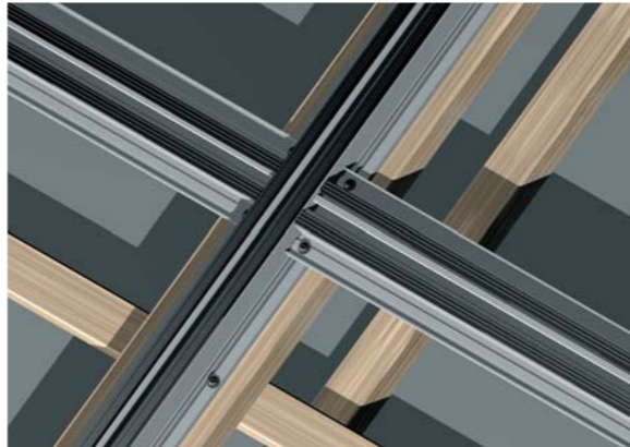
d Installation of the mounting gaskets The mounting gaskets that will later support the laminates are installed into the aluminum profiles.
